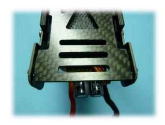
Then shift the bearing plates until the hangers, when inserting the plate for the accumulator, snap in without being forced. Thereafter tighten the 4 pcs M2,5x12 cyl. head Allen screws.
