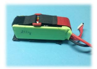
The plate for the accumulator is designed in that way that the accumulator can be fixed longitudinal or at right angle by means of Velcro tape or shrink sleeving.
