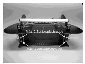
III. 8 M4x12 countersunk screw M4x8 countersunk screw
